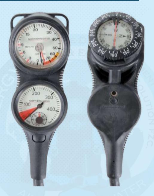
A 2 + 1 console incorporating 450 bar contents gauge with built-in thermometer, 80 metre MDI\* depth gauge and a rotating bezel compass mounted on the back. Hose length 32"/81cm. 63mm face size.
